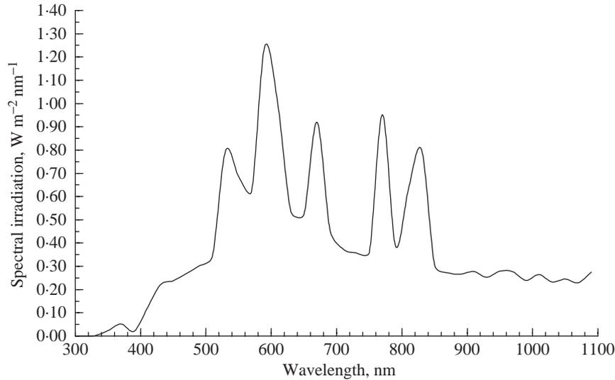
Fig. 3. Measured spectral distribution of the lamp irradiation in the solar simulator at the Technical University of Denmark; radiation level on the top glass surface of the experiment roof module
