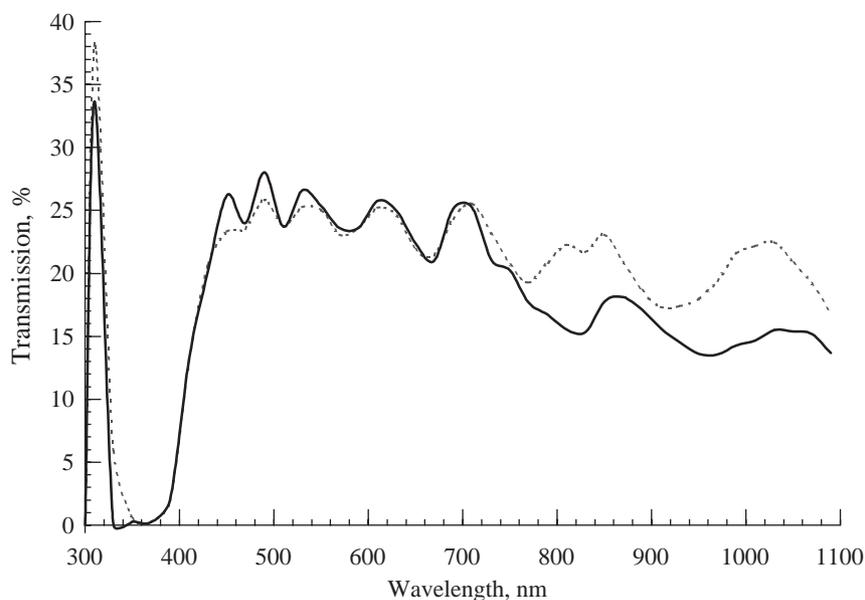
Fig. 5. Measured spectral transmission in the solar simulator for the complete roof with and without water flow on the absorber; the glass thickness is 4 mm and the water layer thickness about 2 mm: ..... , without flow; —, with flow
