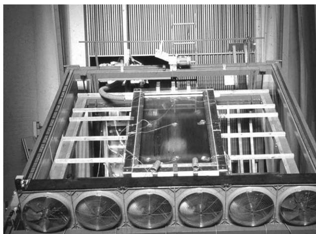
Fig. 2. Laboratory experiment with solar desalination module
