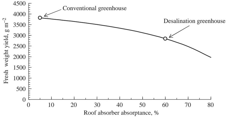
Fig. 8. Simulated seasonal lettuce crop yield as a function of absorber absorptance in Tunisian winter climate. Variation of the absorber absorptance between 5 (left) and 80% (right); asymmetrical greenhouse roof with 26° slope and low quality glass
