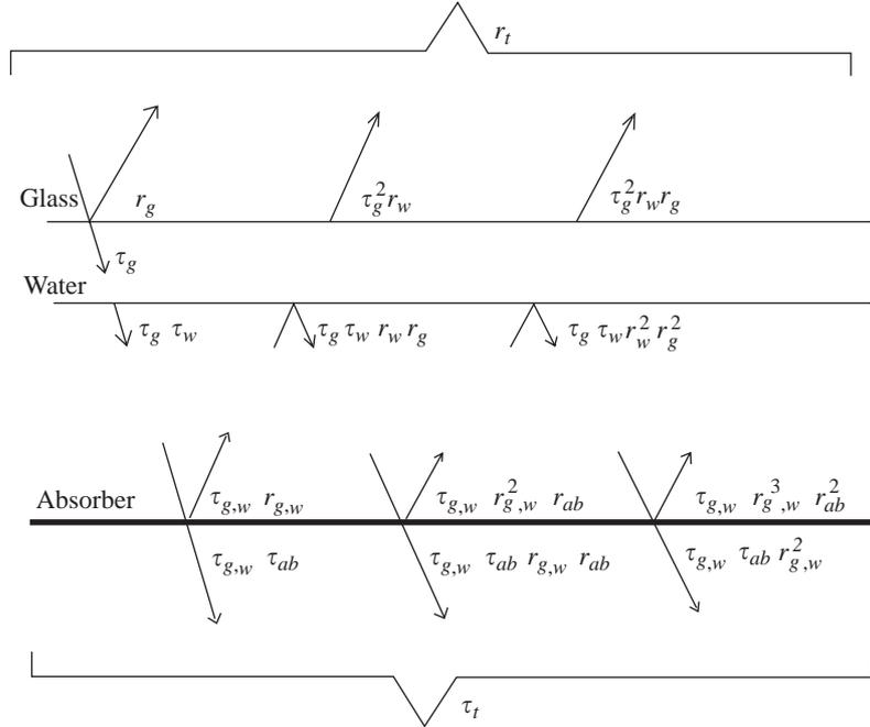
Fig. 4. Principal calculation of radiation transmission components with regard to absorption and multiple reflections in the glass, water and absorber layer of the roof:  $\tau_t$ , the total roof transmission for a specified wavelength interval;  $r_i$ , the total reflection for a specified wavelength interval; subscripts  $g,w$  and  $ab$ , glass, water and absorber layers
