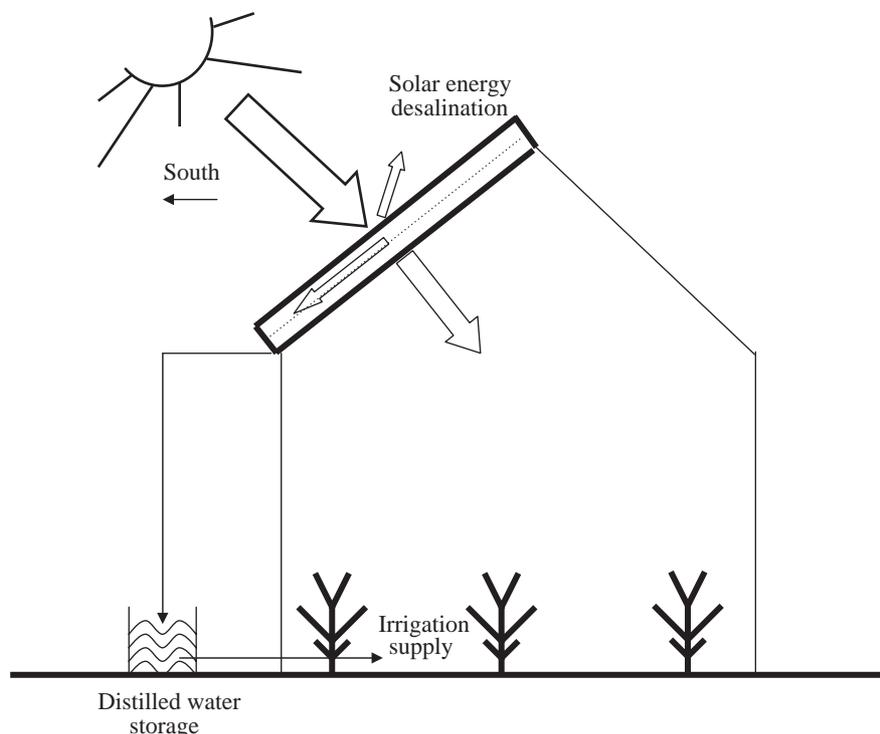
Fig. 1. Principle of a water desalination system integrated in a greenhouse roof
