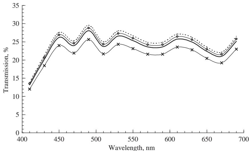
Fig. 6. Simulated compared to measured transmission of photosynthetically active radiation (PAR) in the solar simulator with water flow on the absorber; variation of the extinction coefficient ( $\beta_g$ ) for the top glass material; the glass thickness is 4 mm and the water layer about 2 mm: —, measured; ..... , simulated ( $\beta_g = 5\text{ m}^{-1}$ ); -○-, simulated ( $\beta_g = 15\text{ m}^{-1}$ ); —×—, simulated ( $\beta_g = 20\text{ m}^{-1}$ )
