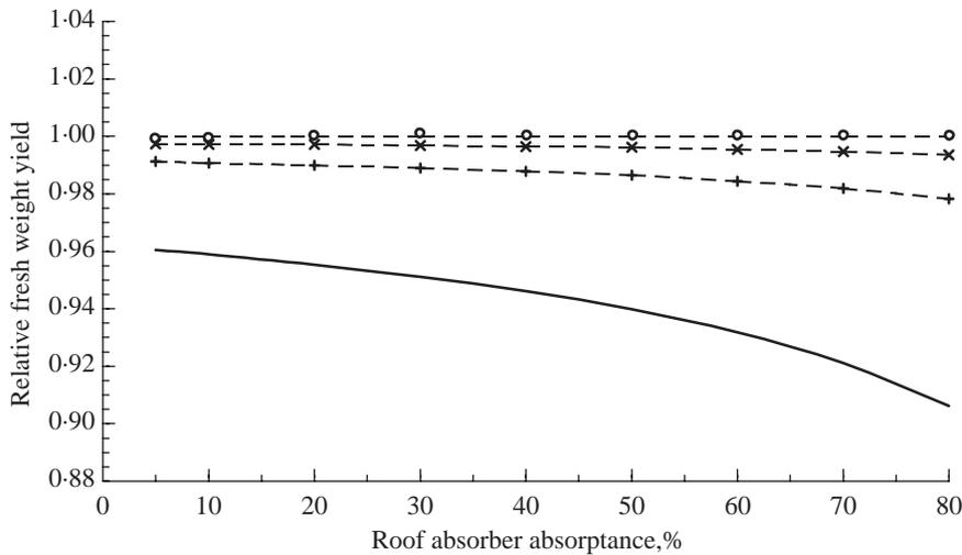
Fig. 9. Simulated relative seasonal lettuce crop yield as a function of absorber absorptance in Tunisian winter climate; variation of the top glass extinction ( $\beta_g$ ) and reflectivity; asymmetrical greenhouse roof with 26° slope; the yield is related to the reference yield ( $\beta_g = 16 m^{-1}$ ) for each specific absorptance level: --○--,  $\beta_g = 4 m^{-1}$ ; --×--,  $\beta_g = 8 m^{-1}$ ; --+--,  $\beta_g = 16 m^{-1}$ ; —,  $\beta_g = 32 m^{-1}$
