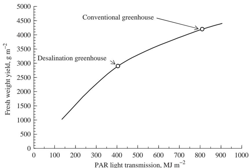
Fig. 7. Simulated seasonal lettuce crop yield as a function of seasonal transmission of photosynthetically active radiation (PAR) (horizontal) in Tunisian climate; variation of the absorber absorbance between 5 (right) and 80% (left); asymmetrical greenhouse roof with  $26^\circ$  slope and low quality top glass
