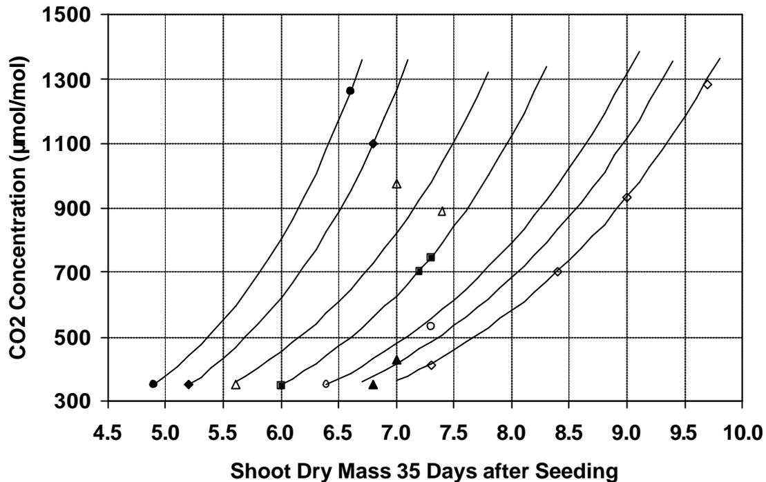
Figure 6. Lettuce (cultivar Vivaldi) shoot dry mass production at 35 days after seeding versus average aerial CO<sub>2</sub> concentration ( $\mu\text{mol}\cdot\text{mol}^{-1}$ ) during the light period. The curved lines indicate the required daily integrated light level ( $\text{mol}\cdot\text{m}^{-2}\cdot\text{d}^{-1}$ ) from 11 through 17  $\text{mol}\cdot\text{m}^{-2}\cdot\text{d}^{-1}$  (in steps of 1  $\text{mol}\cdot\text{m}^{-2}\cdot\text{d}^{-1}$  from left to right).
